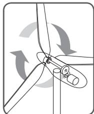
Mechanical (rotation) to Electrical: Inside the wind turbine's housing is an electrical generator. The spinning shaft turns a set of magnets mounted on a rotor. These magnets cause an electrical current to flow in a set of tightly wound coils of wire, located close to the moving magnets. This is electricity moving in the wires.
